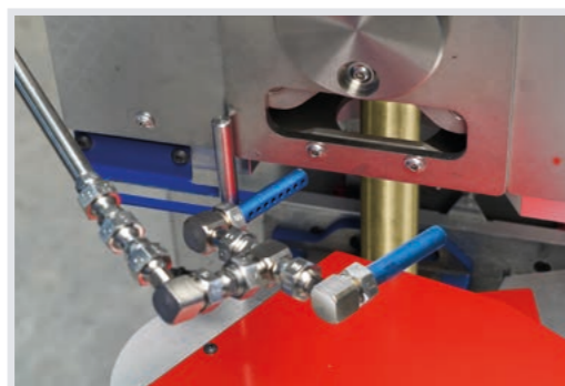
Secondary cooler at the outlet
