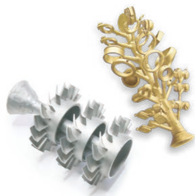
Casting trees in steel and in gold
