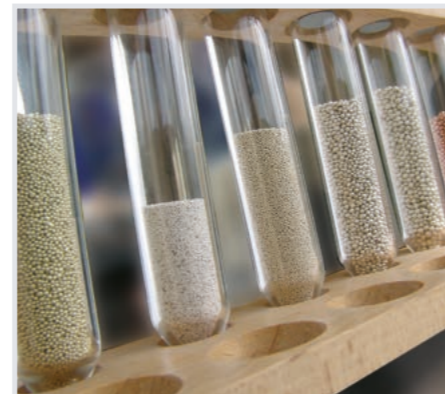
Micro granules in different alloys with a grain size of between 0.1 and 1 mm.
