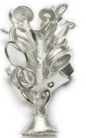
A significant cost factor is the small amount of metal that must be calculated for the sprue.
