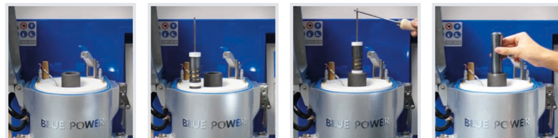
For sintering, the individual layers are centered on a spindle. For the simultaneous processing of multiple rings, the rings are separated by graphite shims.
